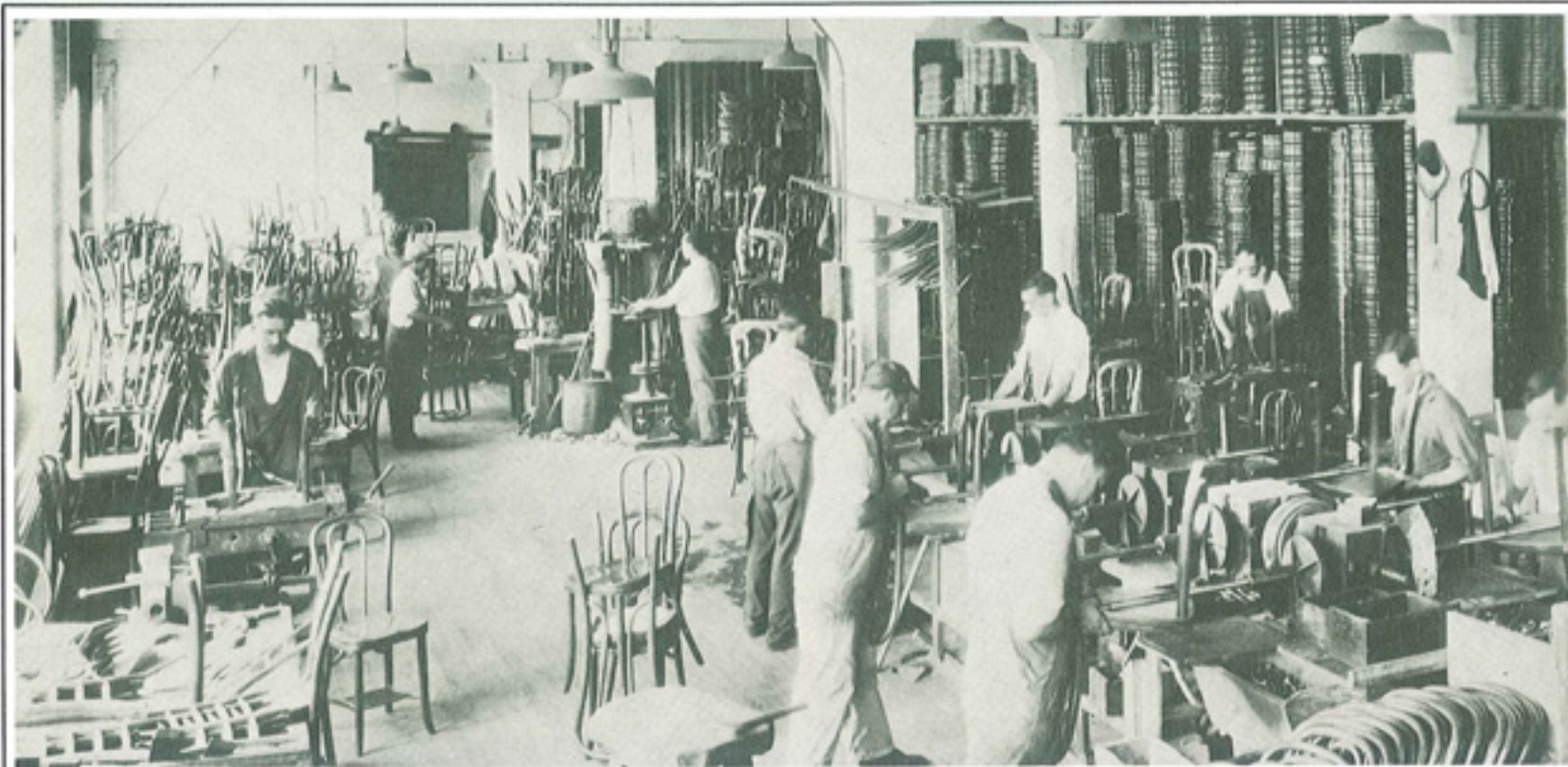
150. Bentwood parts shipped from Europe are assembled at Thonet's Long Island City factory during the 1930s.
